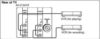
When you use VIDEO-1 INPUT, you should choose to connect S-VIDEO or video input. If S-VIDEO connector and video input are connected at the same time, no picture display on the screen and the message "PLEASE DISCONNECT VIDEO-1 CABLE!" appears. In this case, you should disconnect either S-VIDEO or video input.
