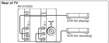
When you use VIDEO-1 INPUT, you should choose to connect S-VIDEO or video input. If S-VIDEO connector and video input are connected at the same time, no picture displays on the screen and the message "PLEASE DISCONNECT VIDEO-1 CABLE!" appears. In this case, you should disconnect either S-VIDEO or video input.
